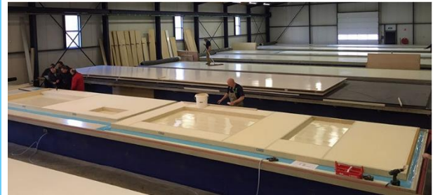
Production of the Cocoonz façade elements for Lekkerkerk demonstration case
