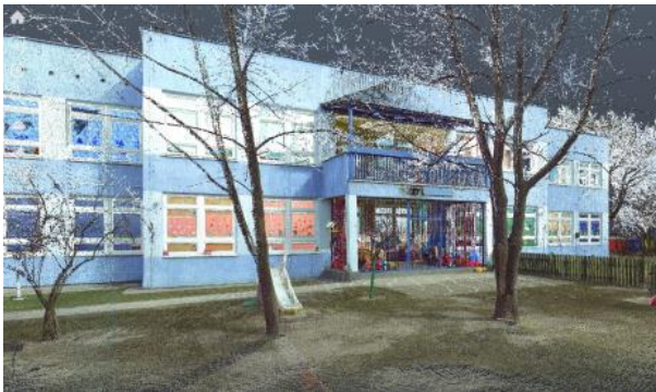
3D Point Cloud from ext. and int. scanning
