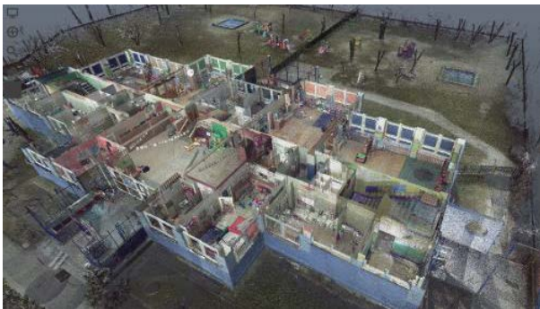
3D Point Cloud from ext. and int. scanning
