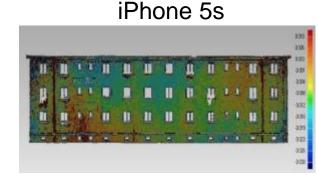
Low-cost cameras show significant noise level in the data - up to several centimeters.
