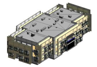
Renovation Design with PnP solutions as prefabricated panels, smart windows and HVAC engine with E-Marketplace and Parametric Modeller.
