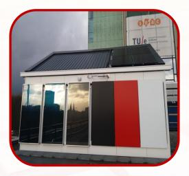
Solar heat collectors based on the usage of NIR absorbing coloured coatings
