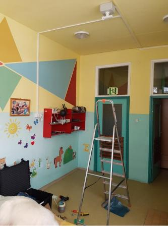
Comfort Eye from Università Politecnica delle Marche for IEQ monitoring and assessment, monitoring thermal comfort according to ISO7730 and IAQ
