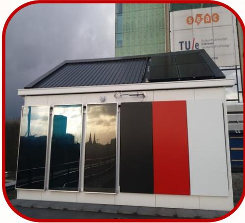
**Solar heat collectors based on the usage of NIR absorbing coloured coatings**
