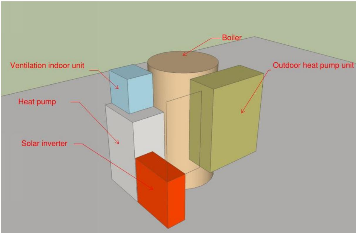
Figure 19: Graphical visualization of all the HVAC components for the Breda residential demonstration case in one 1m<sup>3</sup> space.
