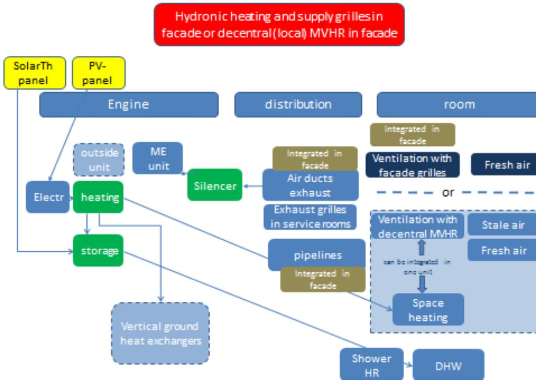
Figure 17: Scheme hydronic heating with decentral ventilation.
