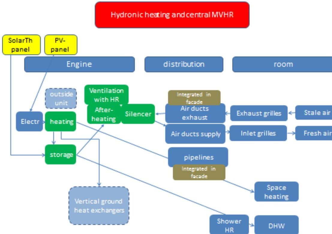
Figure 16: Scheme hydronic heating with central mechanical ventilation and heat recovery (MVHR).
