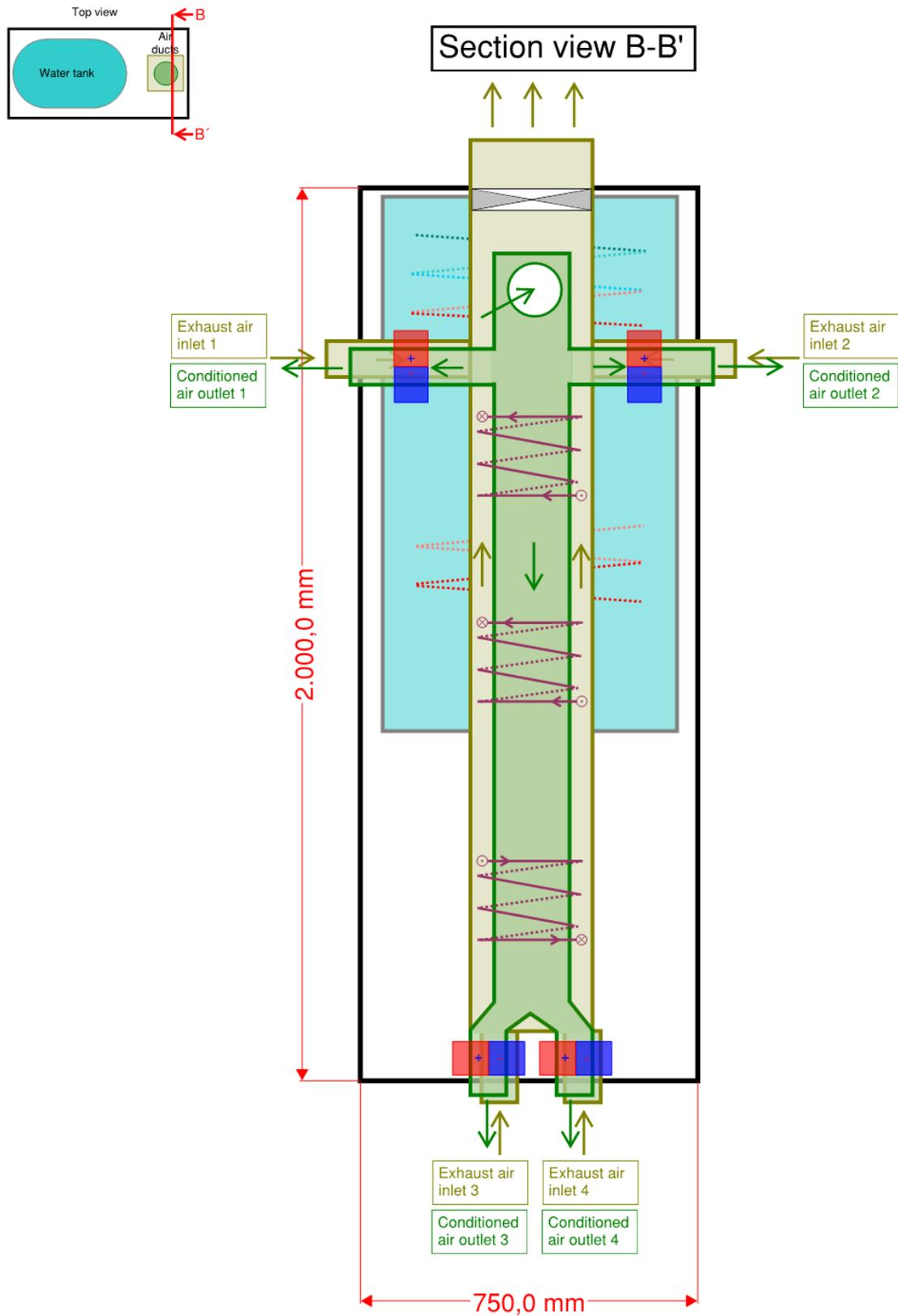
Figure 23: Side section of the HVAC engine for the Breda demonstration case.
