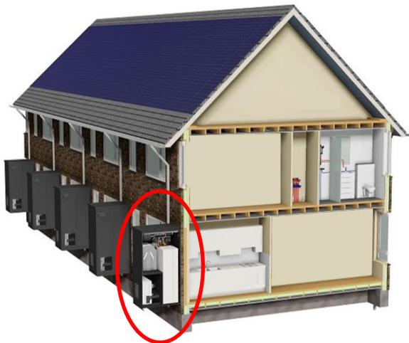
Figure 10: Schematic picture of a prefab renovated single family dwelling with engine next to front door.
