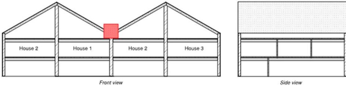
Figure 32: Single P2Endure Engine unit used to satisfy HVAC needs for the 2 neighbouring houses (adjacent walls).
