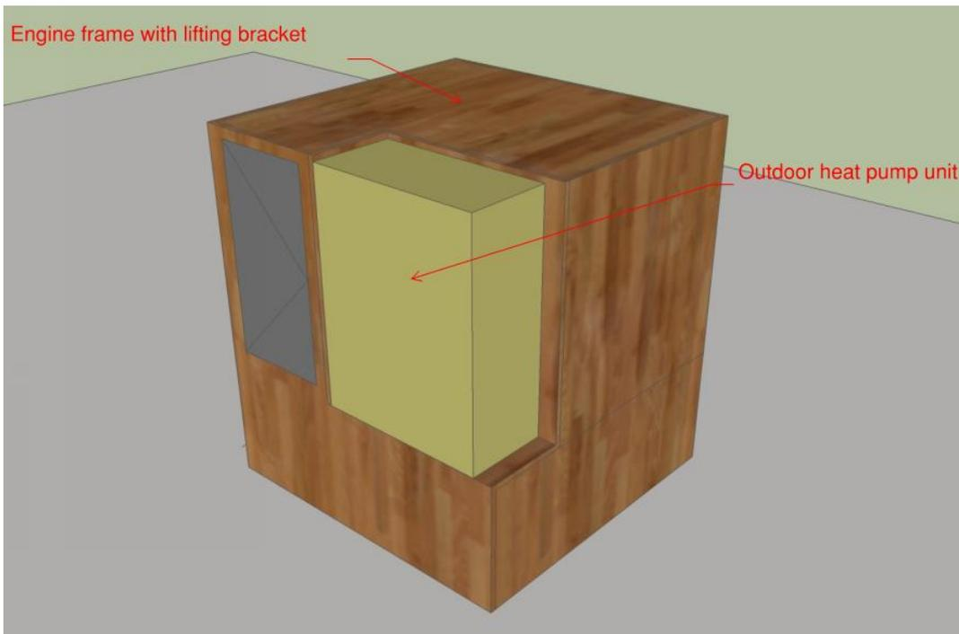
Figure 20: Graphical visualization of the HVAC Engine for the Breda demonstration case.
