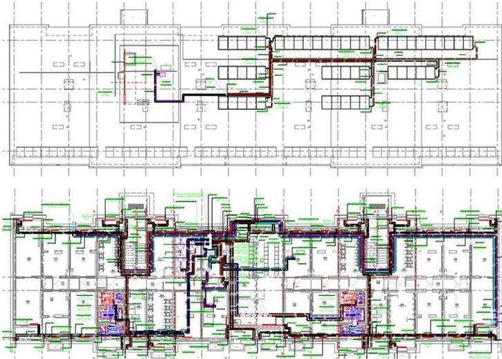
Figure 35: Prefabricated installation platforms for ventilation and DHW, Estonian demonstration building, MORE-CONNECT
