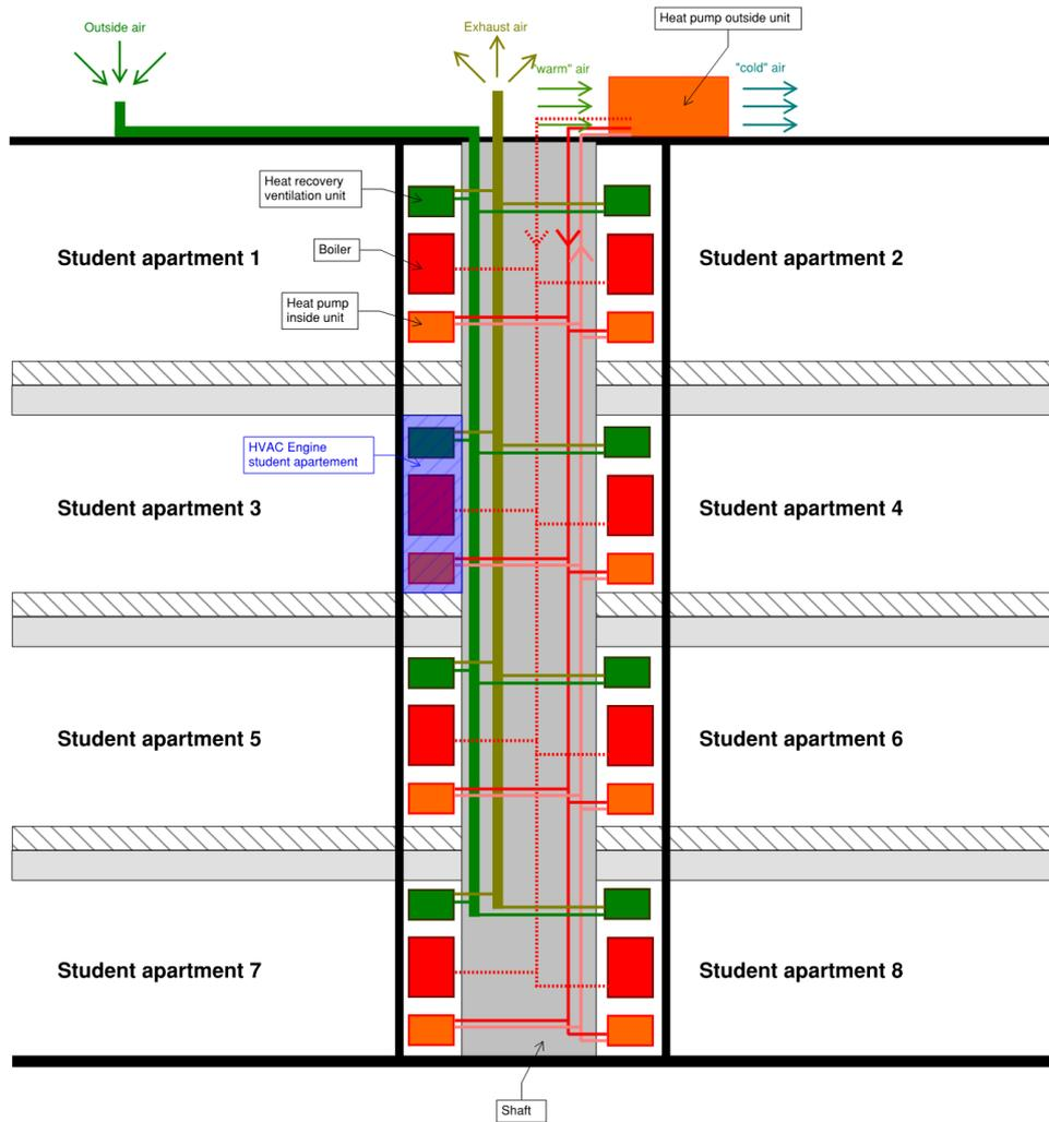
Figure 30: The HVAC engine concept developed for the student housing.
