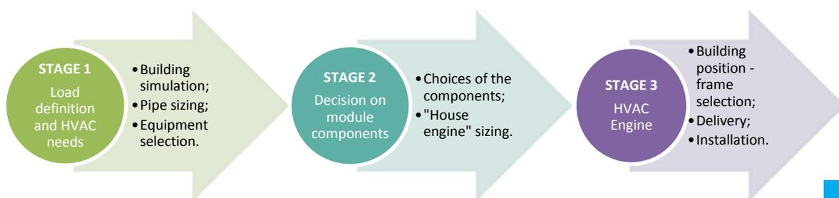
Figure 2: A 3-step guide to design a modular HVAC engine.
