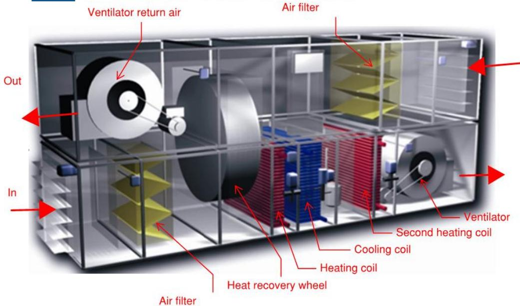
Figure 27: Example of a stand-alone AHU unit for commercial buildings.
