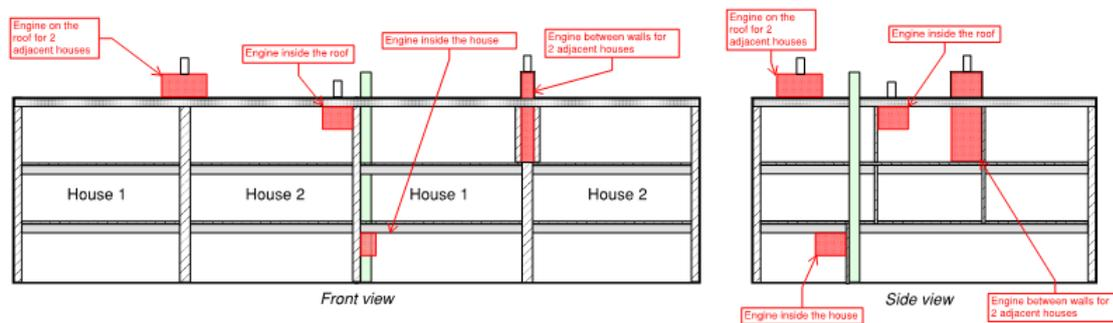
Figure 31: Possible locations of P2Endure Engine for the semi-detached houses.
