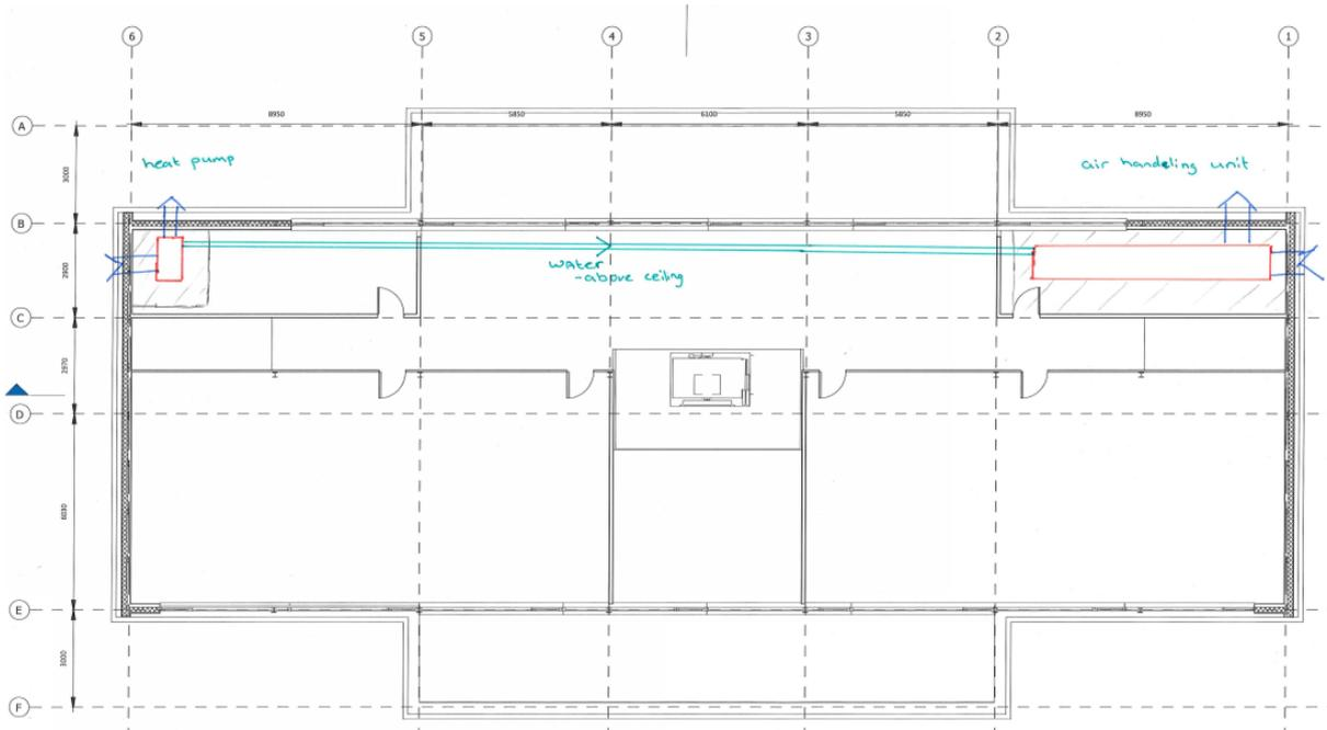
Figure 28: Position of the heat pump and air handling unit for the utility building.
