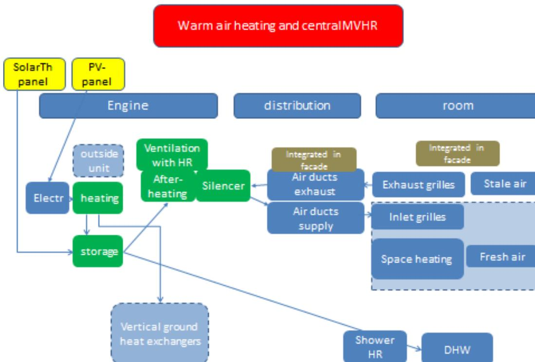
Figure 18: Scheme warm air heating with central mechanical ventilation with heat recovery (MVHR).
