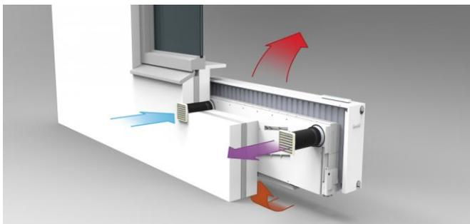
Figure 7: Example of decentral MVHR unit combined with a radiator, CO<sub>2</sub> controlled where no ducts are necessary.
