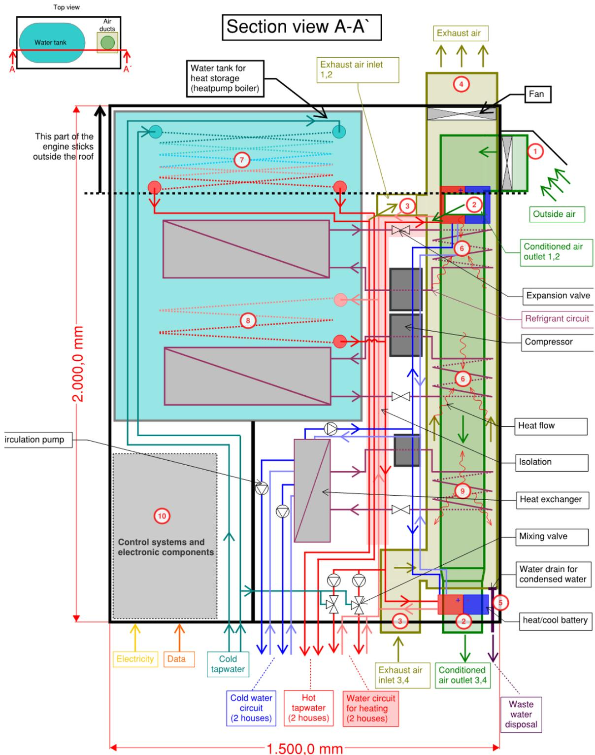
Figure 22: The front and the side section view of the developed integrated HVAC engine design concept developed for the P2Endure Breda demonstration case.
