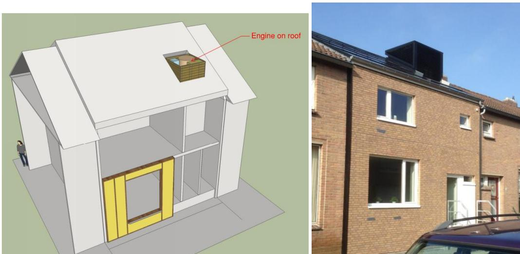
Figure 21: HVAC Engine Sketch-Up model located on the roof (left) and in real life environment (right).
