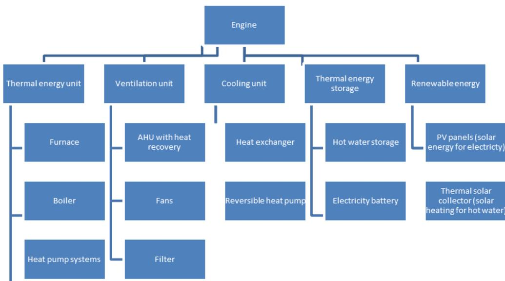
Figure 3: Engine diagram and decision for specific units depends on the building requirements, units related to heating, ventilation, cooling and renewable energy production and storage.
