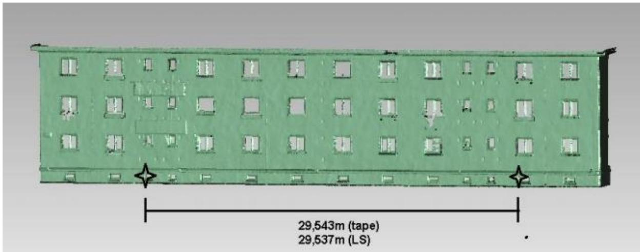
Figure 24: Side measure (source: More-Connect D4.1)
