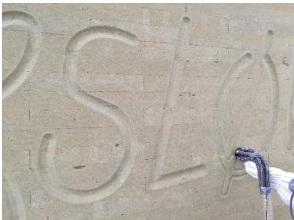
Figure 40: Robot doing design milling
