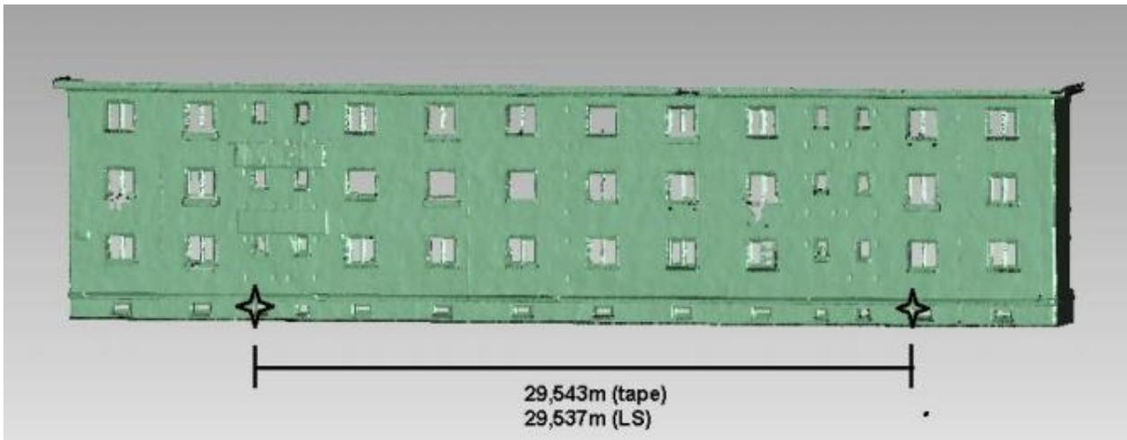
Figure 24: Side measure (source: More-Connect D4.1)
