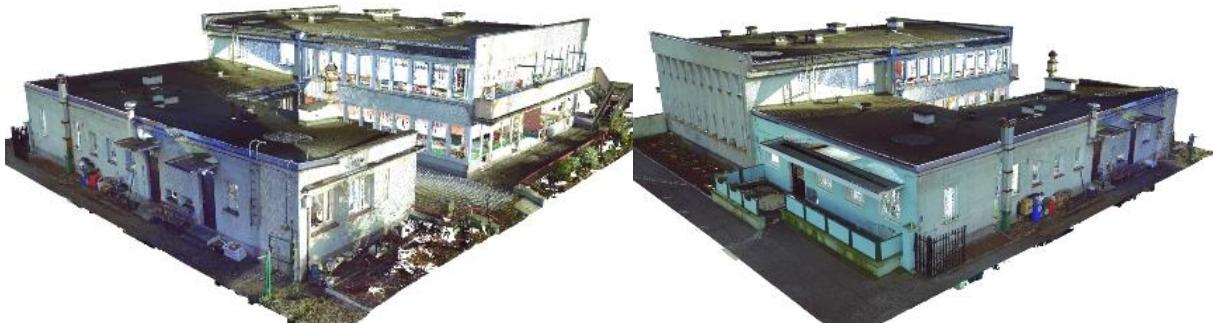
Figure 14: Point cloud model obtained from laser scanning process for Gdynia demo case.
