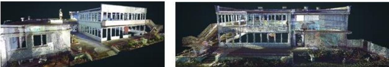
*Figure 7: Point cloud generated from laser scanning in the pilot case of Gdynia*
