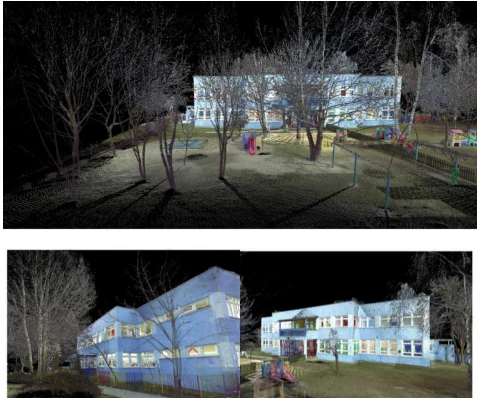
Figure 12: Point cloud model obtained from laser scanning process for Gdynia demo case.
