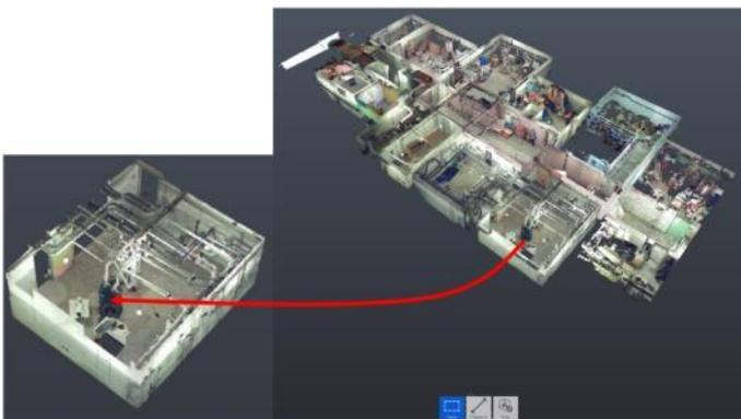
Figure 19. Isolation of area of interest from point cloud.
