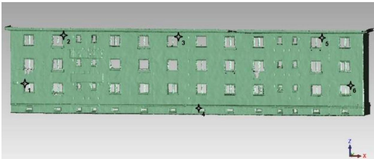
Figure 27: Position of GCP (Source: More-connect D4.1)
