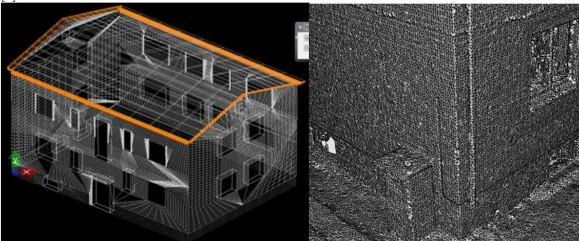
Figure 30: The Smart Surface model of the building generated with Bentley software (left) and the triangulated surface of the corner of building walls generated with 3DReshaper software (right) [8].
