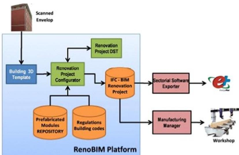
Figure 33: RenoBIM tool Architecture [10].
