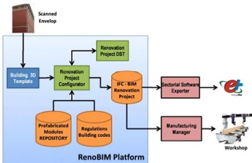
Figure 33: RenoBIM tool Architecture [10].
