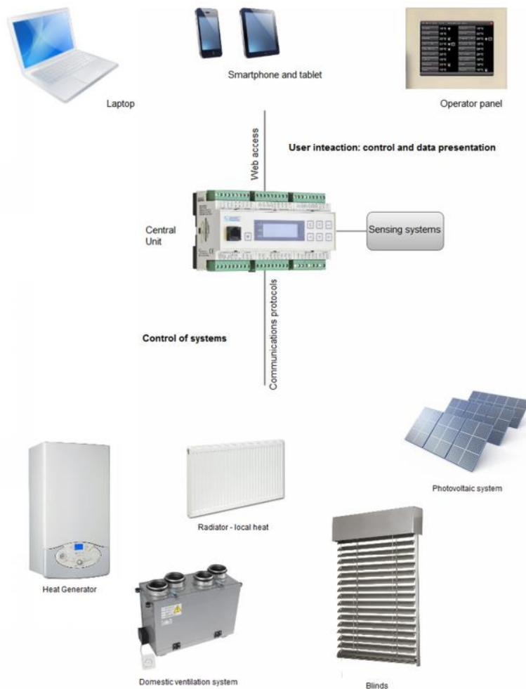
Figure 38: Illustrative diagram for user control of diverse systems [8]
