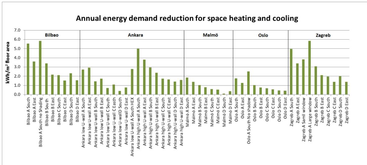
Figure 18: Annual energy demand reduction due to the installation of new A2PBEER smart windows.
