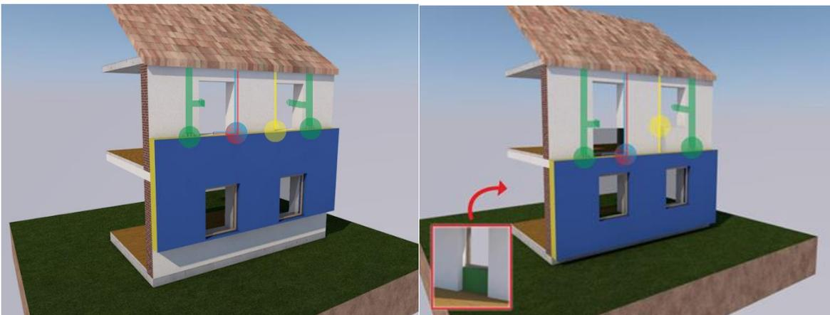
*Figure 2 (left): Optimal position of modules in situation when in the external wall are windows with parapets that cannot be removed and the opening cannot be enlarged. Pipes of the heating system are connected beneath the window sill.*
