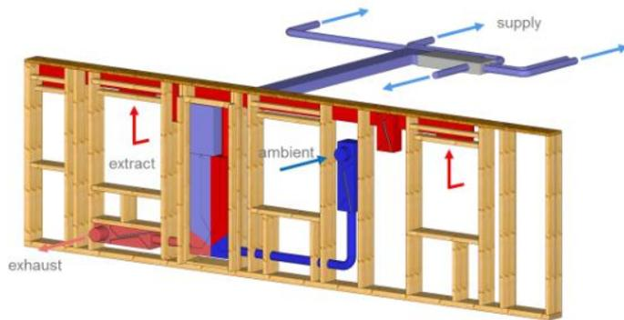
Figure 15: Diagram explaining the concept of the MVHR system with the integrated micro heat pump [15].
