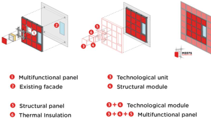
Figure 12: MeeFS concept: A Multifunctional Energy Efficient Façade System for Building Retrofitting [14].
