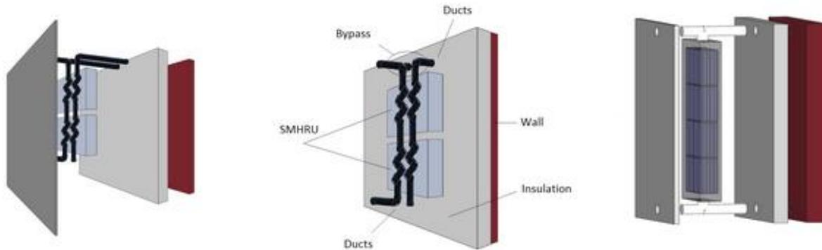
Figure 7: E2vent system (left), Smart Modular Heat Recovery Unit (SMHRU, middle) and Latent Heat Thermal Energy Storage (LHTES, right) [12].
