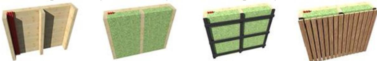
Figure 6: Development of the BERTIM prefabricated building envelope module [10].
