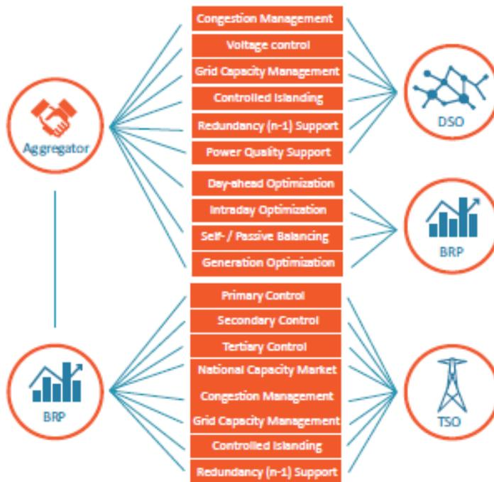
Figure 43: Added business cases. On the up, relation between prosumer and aggregator that aggregates flexibility and sells it to the BRP, DSC or TSO. On the bottom; overview of all possible cases via which an aggregator can create value from flexibility [34].
