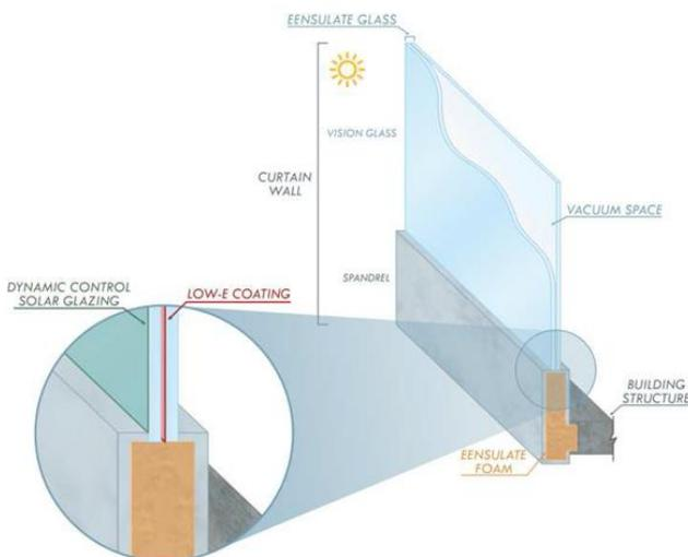
Figure 8: Scheme of the EENSULATE technology for high performance curtain walls [13].
