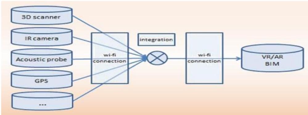
Figure 31: Data integration with a cloud based Building Information Model (BIM) [22].
