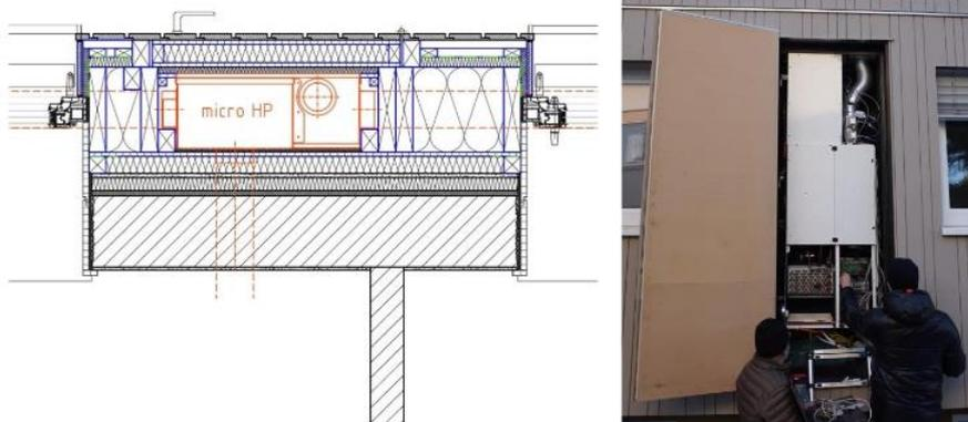
Figure 14: Detail section of the integration of the micro heat pump with MVHR (mechanical ventilation with heat recovery) unit (left) and picture of the installed unit (right) for the demonstration case in Ludwigsburg, Germany [15].
