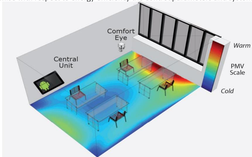
Figure 35: Scheme of the low-cost sensor, *Comfort Eye*, for the monitoring of thermal comfort in indoor environments [26].
