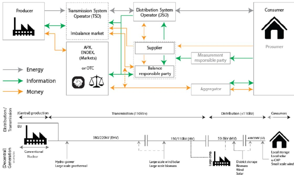
Figure 42: Top - classic physical system with new decentralized producers included.
