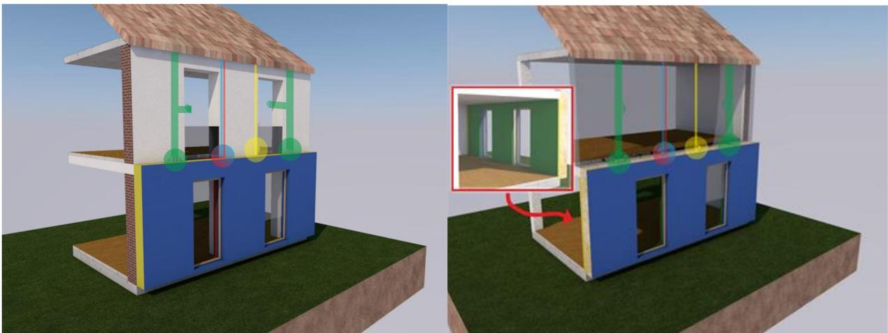
Figure 4 (left): Optimal position of modules in situation when two French windows are required by the design.
