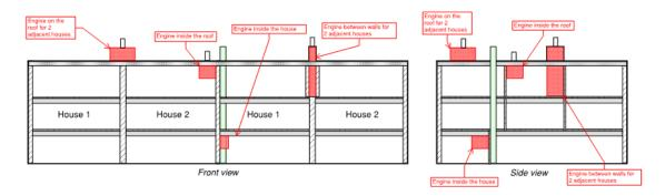
Figure 31: Possible locations of P2Endure Engine for the semi-detached houses.
