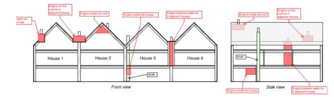
Figure 25: Different location possibilities for the HVAC engine placement.
