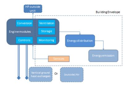
Figure 15: Schematic overview of modules needed in an engine.
