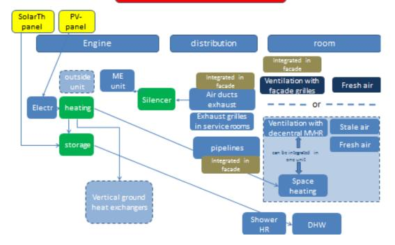
Figure 17: Scheme hydronic heating with decentral ventilation.
