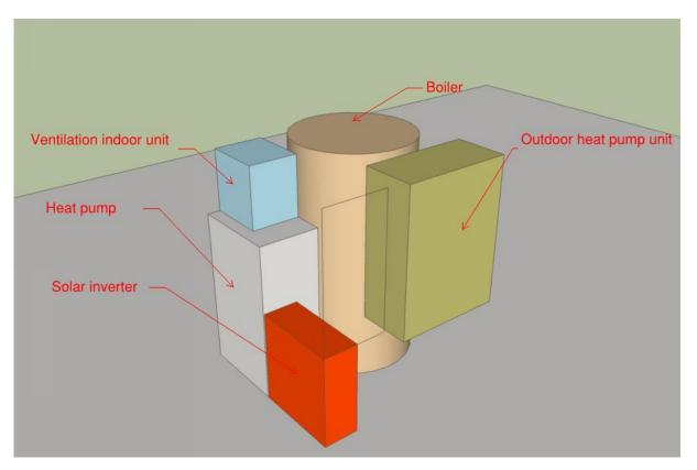
Figure 19: Graphical visualization of all the HVAC components for the Breda residential demonstration case in one 1m3 space.
