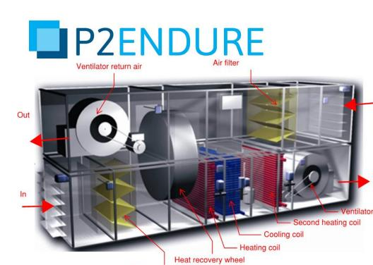
Air filter Figure 27: Example of a stand-alone AHU unit for commercial buildings.
