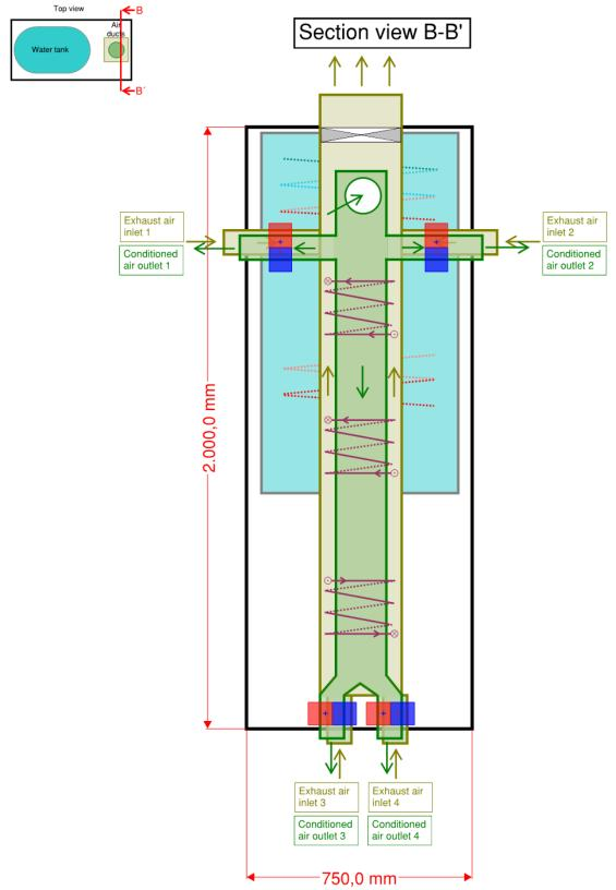
Figure 23: Side section of the HVAC engine for the Breda demonstration case.
