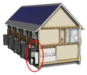
Figure 10: Schematic picture of a prefab renovated single family dwelling with engine next to front door.
