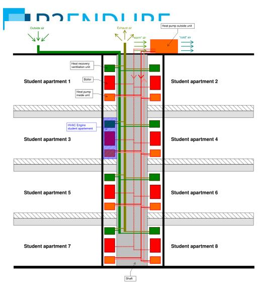
Figure 30: The HVAC engine concept developed for the student housing.
