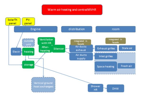
Figure 18: Scheme warm air heating with central mechanical ventilation with heat recovery (MVHR).
