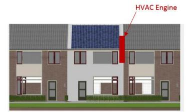
Figure 24: Example of the HVAC engine placement for the Breda demonstration case.
