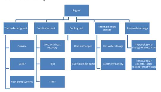
Figure 3: Engine diagram and decision for specific units depends on the building requirements, units related to heating, ventilation, cooling and renewable energy production and storage.
