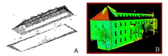
Figure 5: Block of flats, perspective view. (A) Aerial laser scanning data (B) Terrestrial laser scanning data (intensity colours).
