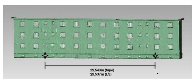
Figure 24: Side measure (source: More-Connect D4.1)
