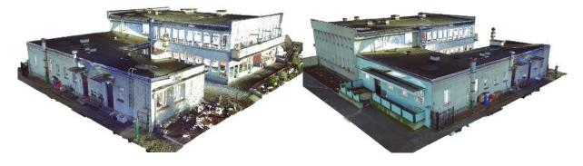
Figure 14: Point cloud model obtained from laser scanning process for Gdynia demo case.
