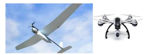
Figure 33: This is two typical UAV, on the left a fixed wing model and on the right a rotary drone.
