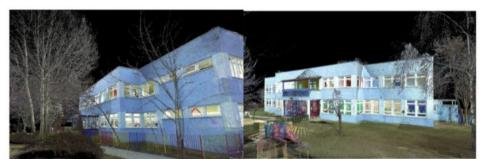
Figure 12: Point cloud model obtained from laser scanning process for Gdynia demo case.
