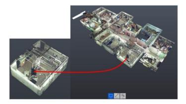
Figure 19. Isolation of area of interest from point cloud.
