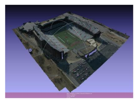
Figure 4: 3D model of Razorback stadium created from four digital aerial images using Photo Scan Pro
