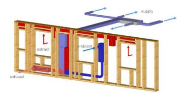
Figure 15: Diagram explaining the concept of the MVHR system with the integrated micro heat pump [15].
