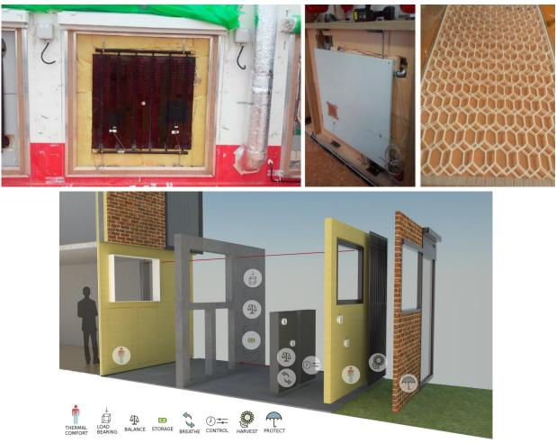
Figure 17: Above - Lab scale prototypes of ADAPTIWALL (left) and prototype of membrane separator (right). Below - ADAPTIWALL concept: The different components of the ADAPTIWALL system [16].
