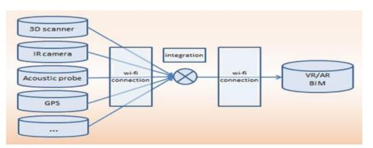
Figure 31: Data integration with a cloud based Building Information Model (BIM) [22].
