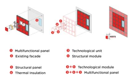
Figure 12: MeeFS concept: A Multifunctional Energy Efficient Façade System for Building Retrofitting [14].
