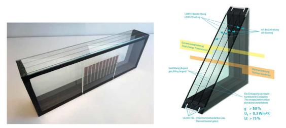
Figure 21: The quadruple IG-unit with Integrated Photovoltaic (left) and section of the novel IG-unit (right) [19].
