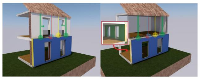
Figure 4 (left): Optimal position of modules in situation when two French windows are required by the design.
