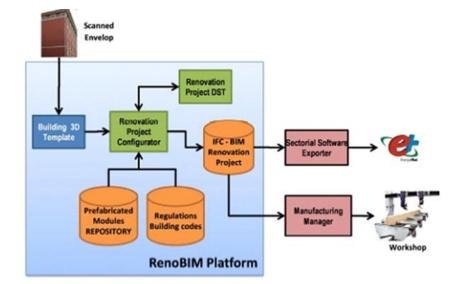
Figure 33: RenoBIM tool Architecture [10].
