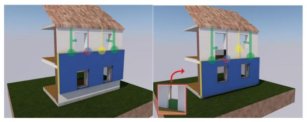
Figure 2 (left): Optimal position of modules in situation when in the external wall are windows with parapets that cannot be removed and the opening cannot be enlarged. Pipes of the heating system are connected beneath the window sill.
