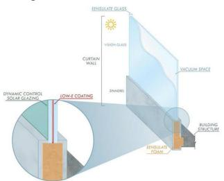
*Figure 8:* Scheme of the EENSULATE technology for high performance curtain walls [13]. P2ENDURE D6.5 State-of-the-art report on innovations for deep renovation
