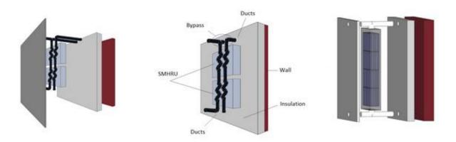
Figure 7: E2vent system (left), Smart Modular Heat Recovery Unit (SMHRU, middle) and Latent Heat Thermal Energy Storage (LHTES, right) [12].
