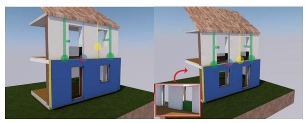
Figure 3 (left): Optimal position of modules in situation when a French window is required by the design.
