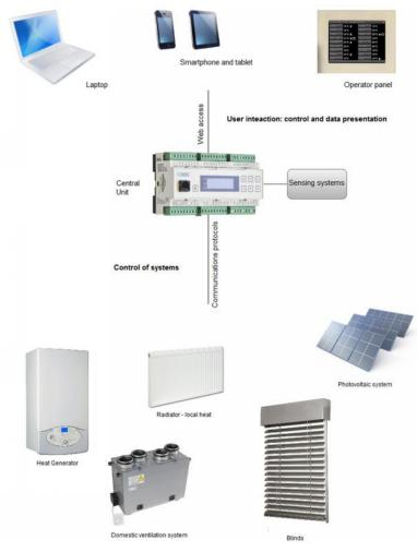
Figure 38: Illustrative diagram for user control of diverse systems [8]
